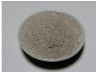
→Carbonate discharged after processing. Can be used as building materials or soil conditioning agents
